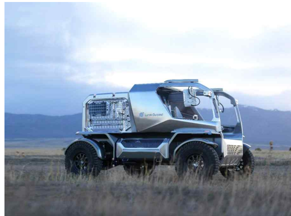
[그림 4-1] A prototype of the Lunar Terrain Vehicle
