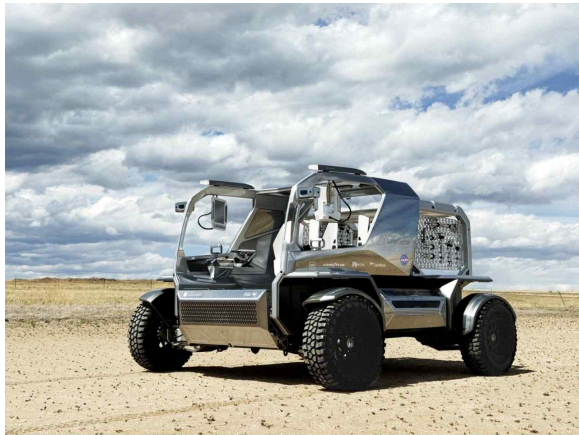
[그림 4-1] A prototype of the Lunar Terrain Vehicle
